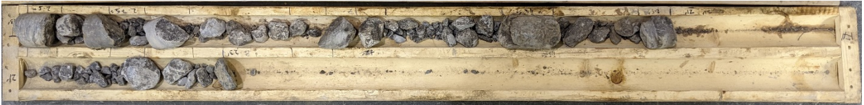
Rock Core from Borehole 4 Run 1: 4.0 to 5.2 metres below grade Run 2: 5.2 to 6.4 metres below grade Run 3: 6.4 to 7.0 metres below grade
