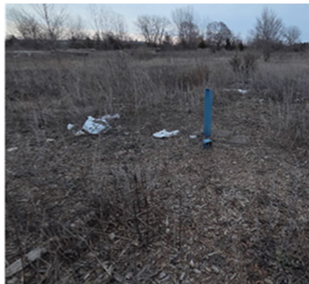
PHOTO 28: View of a destroyed monitoring well located in the field west adjacent to the Phase One Property, facing south.
