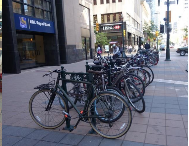
Not so Good = bikes within the pedestrian clearway, and not aligned with other street furniture
