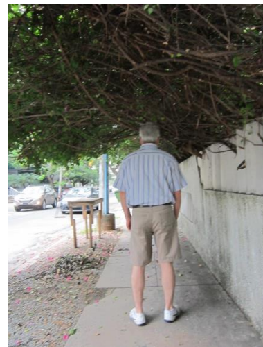
Not so Good = head hazards over the pedestrian clearway
