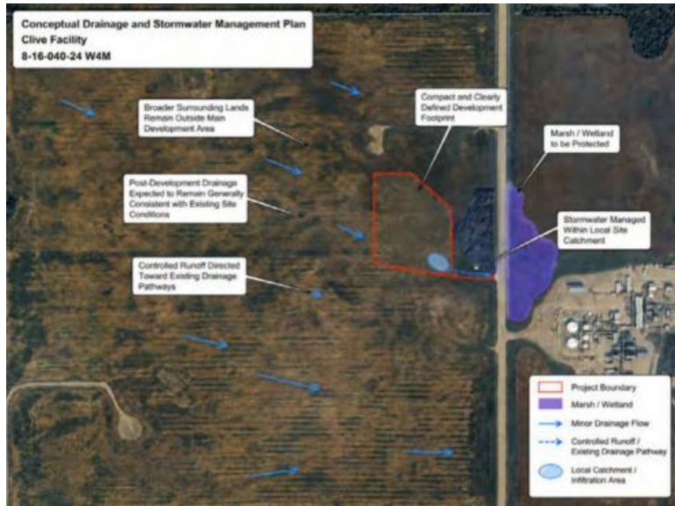
Figure 7: Conceptual Drainage and Stormwater Management Plan
