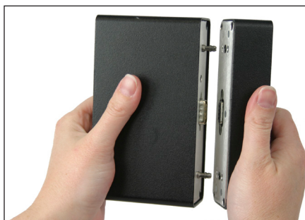
Figure 2.1a Separating the computer/display unit.
