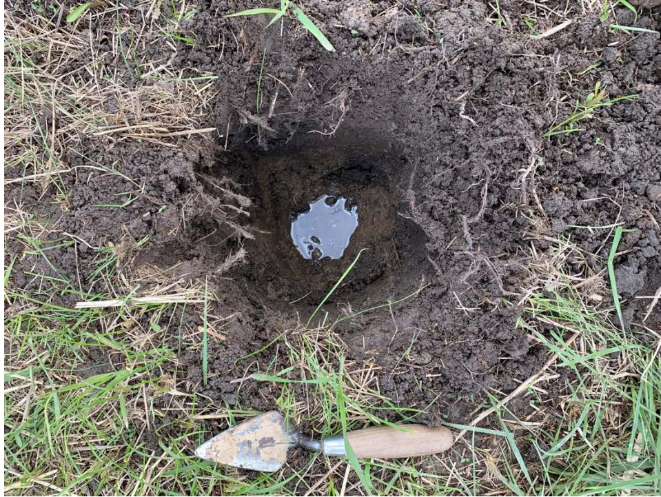
Image 29: Test pit showing low and wet conditions (Trowel pointing North).
