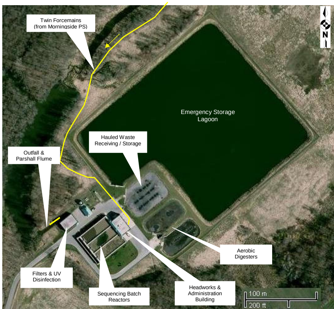
Figure 1.9: New Hamburg WWTP Aerial View
