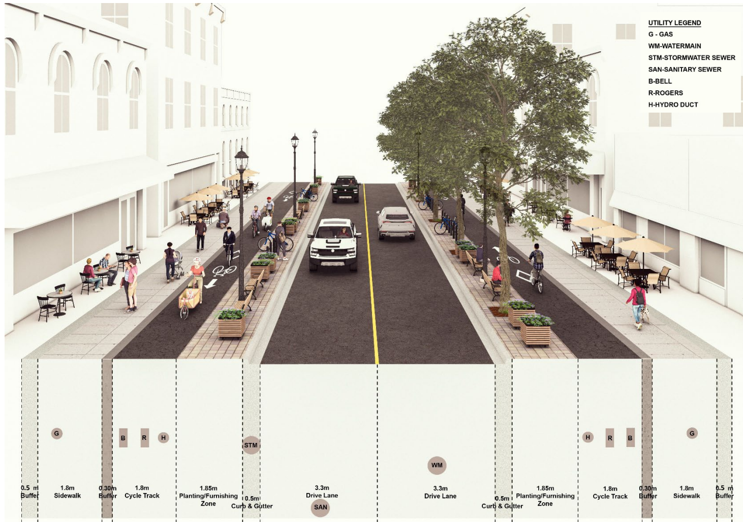
Figure 4.11: Proposed Cross-Section for Case Study #2 - Urban Main Street - 20 m ROW
