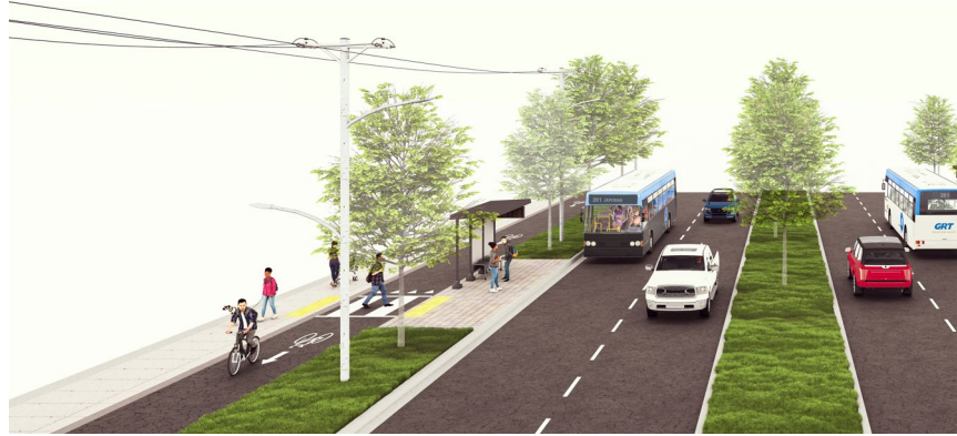
Figure 5.2: Island Boarding Stop on Urban Connector
