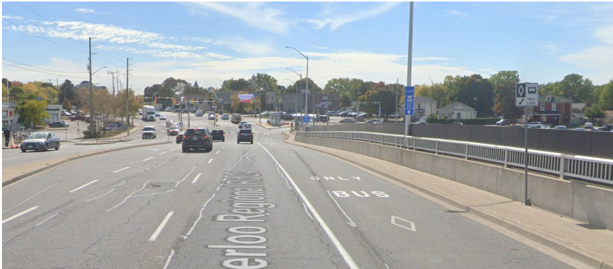
Figure 3.8: Curbside Bus Lanes on Hespler Road Approaching Coronation Boulevard (Source: Google Maps, 2025)
