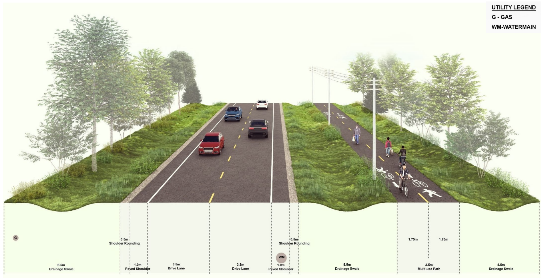
Figure 2.10: Rural Connector — Example 1 (Multi-use Path)— 30 m ROW
