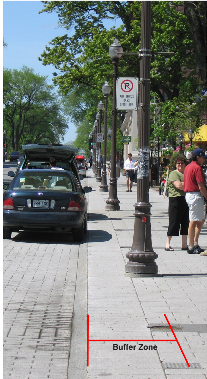
A buffer zone is a street feature, which is used to minimize street clutter and assist with snow storage.
