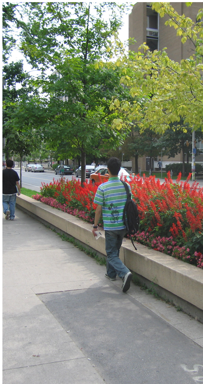
The landscaping and site furnishing zone provides a buffer between the pedestrian clearway and traffic.
