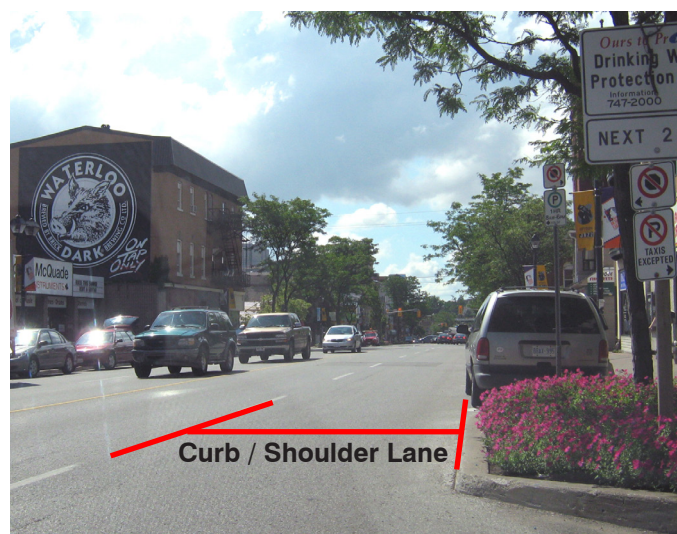
Curb / Shoulder lanes provide for the movement of vehicles travelling from one destination to another, not including shoulders and auxiliary lanes.
