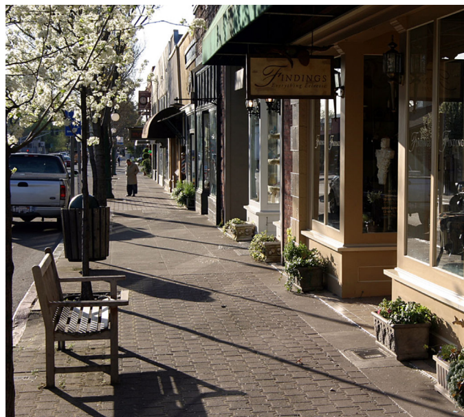
The pedestrian clearway provides a continuous zone that is protected from vehicular traffic.
