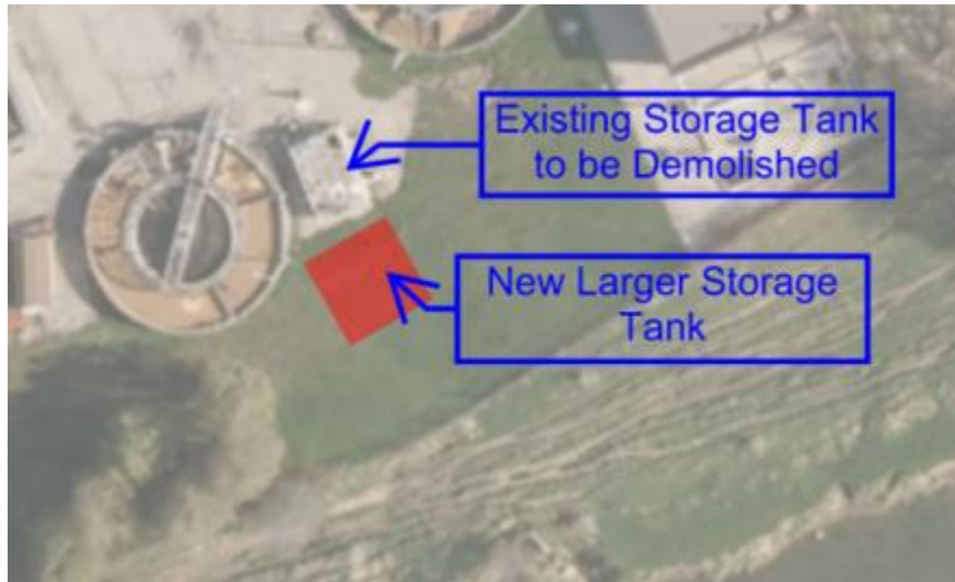
Figure 3-12. Expansion of Existing Sludge Storage Tank
