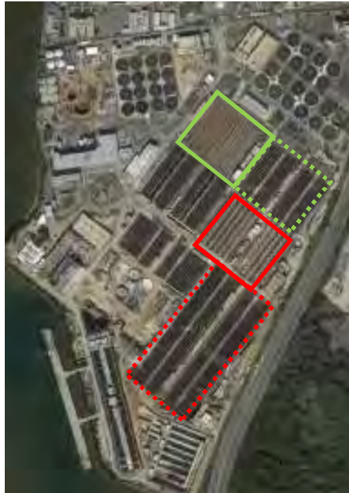
Figure 4-7 Blue Plains WWTF Aerial Photo Showing A-side HRAS Bioreactors (solid green box) and Clarifiers (dashed green box) and the B-Side Nitrification/Denitrification Bioreactors (solid red box) and Clarifiers (dashed red box) (adapted from Stinson et al., 2013)
