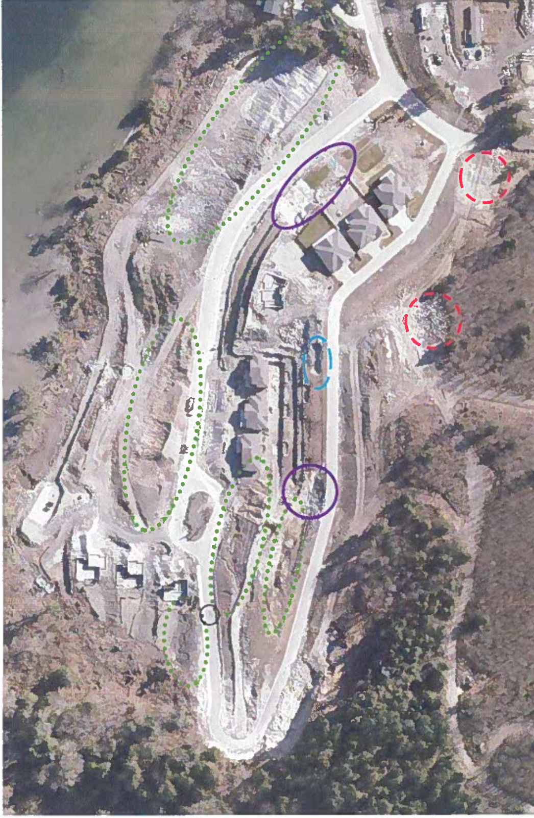
Photo 11. March 2009 image showing signs of recent instability (solid purple lines), springs and/or erosion features (green dotted lines) and significant ground disturbance (red dashed lines). Note that the scarp-like feature is visible at the southeast corner of Lot 21 (blue long dashed line). A small patch in the asphalt surfacing is visible adjacent to Lot 15. Image provided by DOS.
