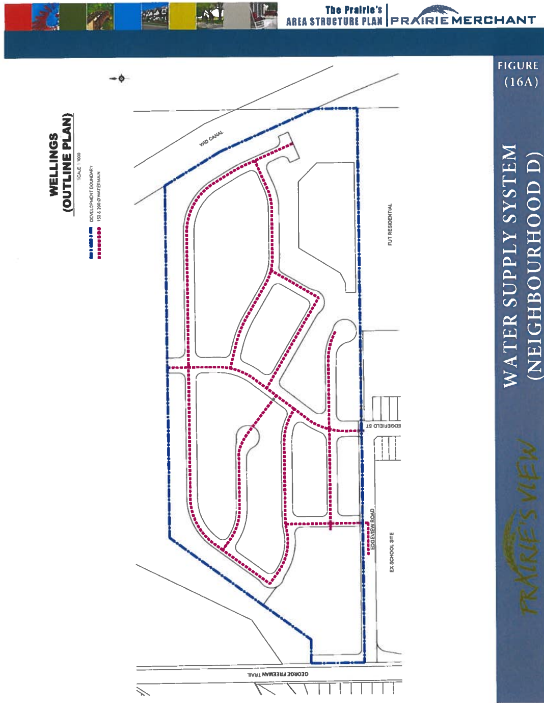
Figure 16a. Water Supply System (Neighbourhood D)
